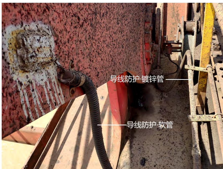
C.10 应变计导线防护图
